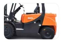
Rigid Transaxle with Shoe Brake The rigid transaxle with shoe brakes includes a 1-speed, powershift transmission and uses a 4-pinion differential bevel gear set to transfer high torque to the drive wheels. The transmission gear is made from carbonized high alloy steel to
