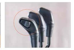
Ergonomically designed hydraulic levers with F/R switch
