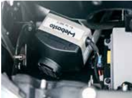
Webasto cabin heater with thermostat, diesel (option)
