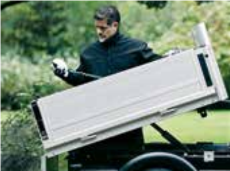
Electric tilting cargo bed with removable drop sides (option)
