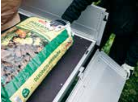
Cargo bed with removable drop sides (option)
