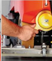
Overview at a glance: Wear indicator for brushes and pads. A comfortable discharge system enables fast and easy changing of the brushes – without the need for tools.
