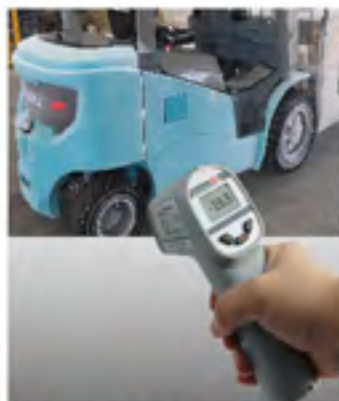
The whole vehicle can be operated alternately in -30°C cold storage for 6 hours and parked in the cold storage for 12 hours without any failure and can continue to work.
